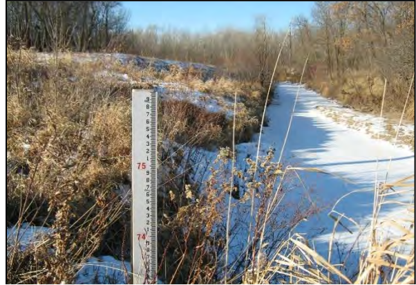
High-water staff gauge – Moose R. at Mar. Co.Hwy. #54
