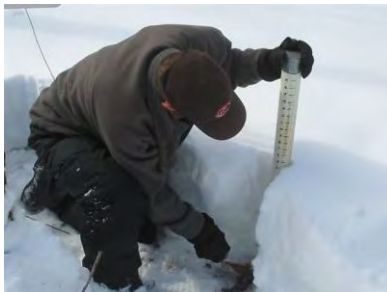
Obtaining snow depth and core sample
