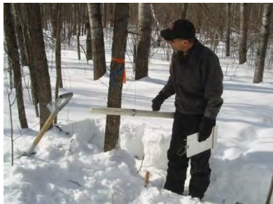
Establish base weight of empty sampling tube
